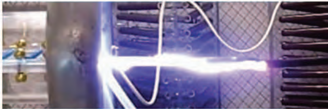
Figure 10. CUT#5. Photo of flashover. Positive polarity.
