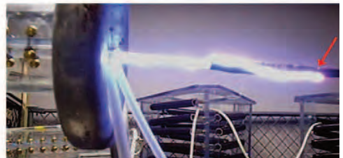
Figure 11. CUT#6. Photo of flashover. Positive polarity.
