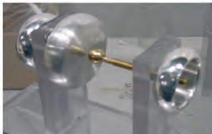
Figure 3. Sphere-to-plane spark gap.
