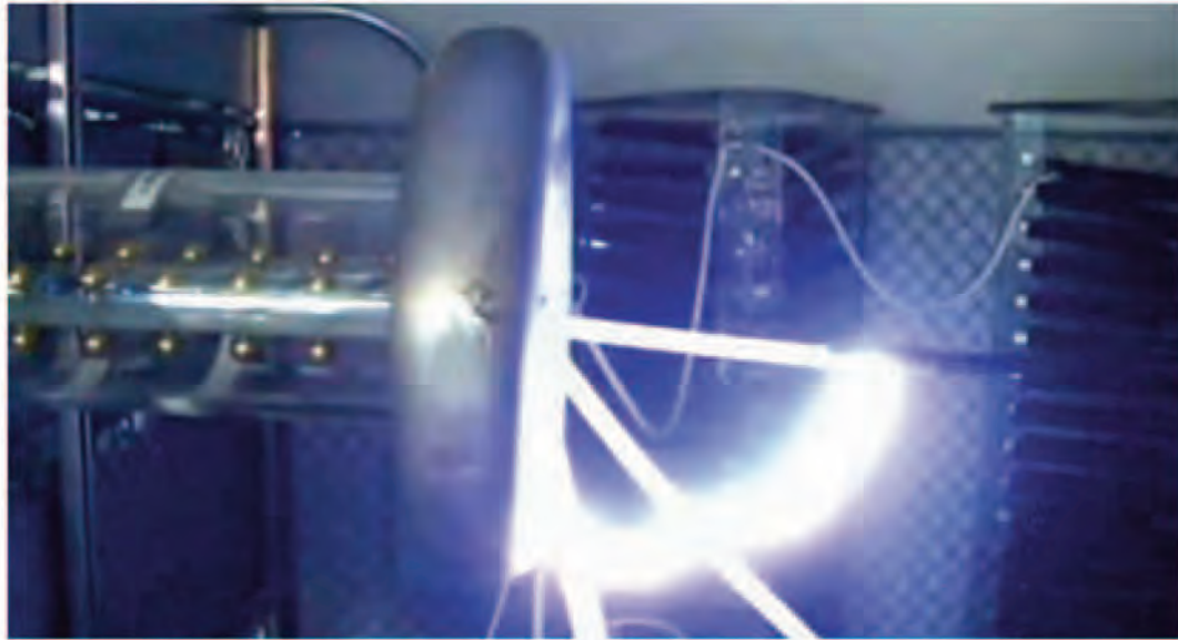
Figure 9. CUT#4. Photo of flashover. Positive polarity.
